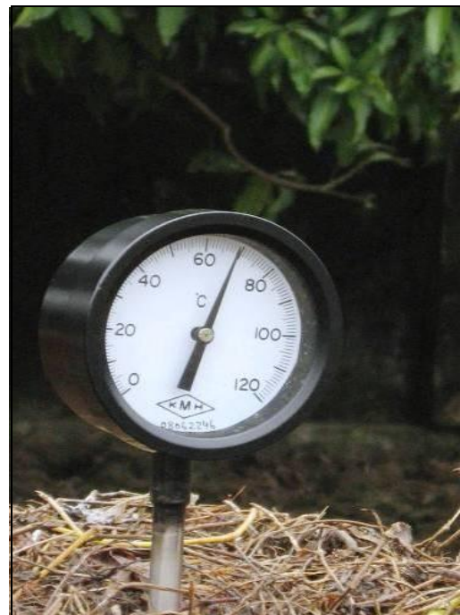
Pic. 13 : Regular monitoring of temperature in Novcom composting heap to ensure compost quality.
