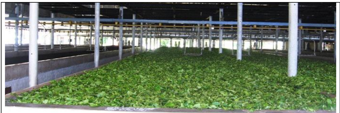
Pic. 92 : Green leaf in weathering turf as part of tea manufacturing process.
